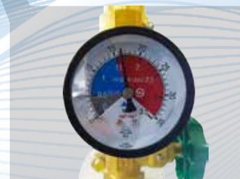
Gas pressure gauge
