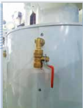
Water overflow valve (Prevent the water evaporation)
